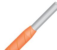
**Tank wall optical feedthrough** Specifically designed for transformer tank walls, this feedthrough has a simple design that provides both toughness and long-term leak-free operation. It is made from 316 stainless steel and relies on proven glass-to-metal bonding techniques. The feedthrough uses 1/4" NPT ANSI threads and can be installed directly into the tank wall or on a tank wall mounting plate. No O-rings are used.
