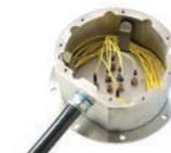
**Tank wall mounting plate & JBox2** Up to 24 feedthroughs can be mounted on a tank wall mounting plate. The plate is made with carbon or stainless steel 316. Tank wall mounting plates can be customized in size or material according to customer specifications, with larger plates allowing more feedthroughs. The mounting plate comes with the JBox2™ protective enclosure.
